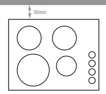
Figure 2: Electric Hotplate clearances
