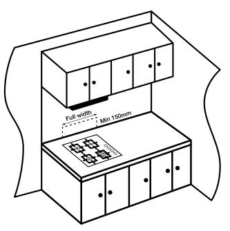
Figure 4: Mark out mineral board position directly behind cooktop and to minimum height of 150mm above the benchtop
