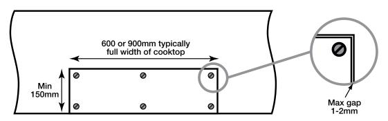
Figure 7: Detailed installation of mineral board with self-tapping screws showing allowable gaps
