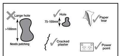
Figure 8: Wall damage and recommended repair requirements
