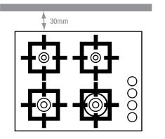
Figure I: Gas Hotplate clearances
