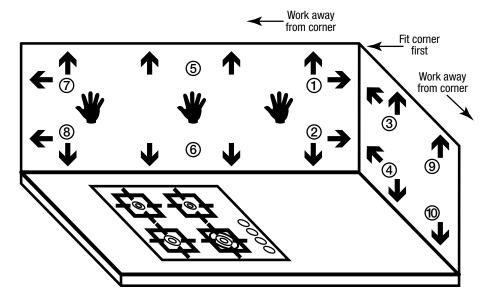
Figure 12: Sequence of panel pressing onto the wall – folded corner method
