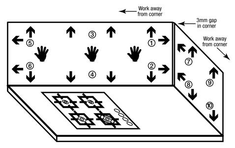
Figure 13: Sequence of panel pressing onto the wall – butt join method
